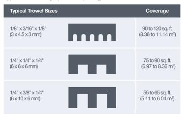
"Trowel dimensions are joint width x depth, x notch space. Coverage depends on substrate condition, tile or stone selected and notched trowel used.
